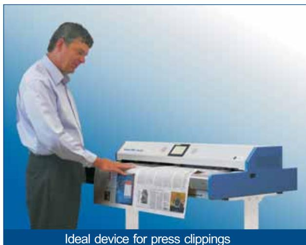
The scanner features two camera boxes, both consisting of three CCD systems, integrated into the upper and lower part of the device. The WideTEK 36 DS captures both sides of the newspaper at the same time. After scanning, software separates the scanned document into four single images; capturing the left and right half of the front and back of the newspaper – everything in one single step.
